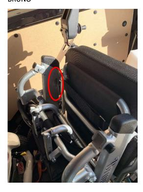
When chair is folded up you will easily find serial number located on the inside of the side frames. It's a bar coded sticker
