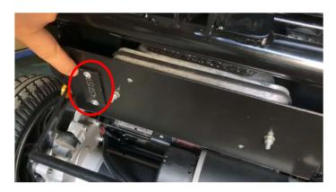
On the bottom of the frame, lift/tilt up from where the footrest is on the powerchair section and there is a plate with number stamped onto it. The full serial number in this instance (as recorded on our system and the customers invoice) is P450159-M480159.
