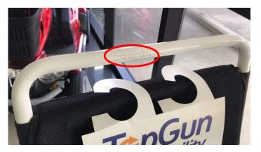
Remove the padding on the back seat framework at the top and the serial number is stamped into to frame
