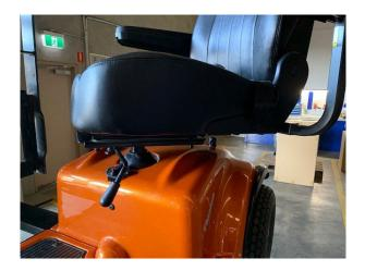
Once the seat is in the 45 degrees position the seat is able to be removed by lifting it straight up
