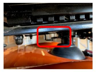
To put seat back onto the scooter, ensure the seat base is at a 45-degree angle when placing seat on post. Once in that position, wiggle the seat slightly to ensure the seat has bottomed out and that you are able to lift the lever on the left-hand side. Once the lever is lifted you can then swivel the seat back to the center position and release the lever ensuring it locks into place.
