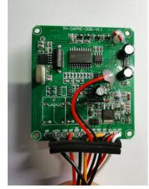
4. Press the remote key to turn on the scooter, and use wires or metal tweezers, make two contacts short circuit like below image, after making sure all good contact, press the lock button of new remote control and unlock button of old remote control
