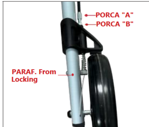
A) Brake tension control system
