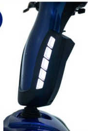
5. Running water turn signal + daytime running lamp
