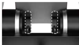
Built-in clutch lever This state is the clutch lever unlocked state. In this state, the wheelchair can be artificially pushed; Joy sticks do not drive wheelchairs. To unlock state: Power off. Put the clutch lever from top to bottom.
